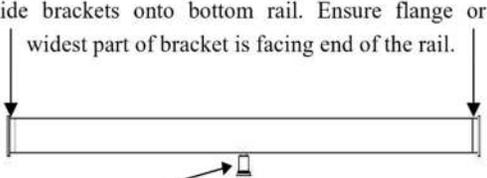
**Note:** Your Premium MAJESTIC Railing does NOT need the foot block with the aluminum in bottom rail! Foot block not included
