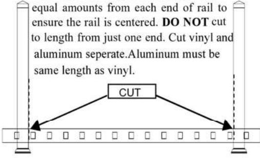
**Note:** Your Premium MAJESTIC Railing does NOT need the foot block with the aluminum in bottom rail! Foot block not included
