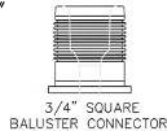
3/4 inch Diameter, 0.045 inch wall, Aluminum Picket
