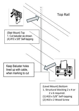
Please note: Begin by inserting screws into the top mount first. Then, Plumb the baluster and insert screws accordingly. Level mount screw holes should be facing inside toward stairs for ease of installing screws.
