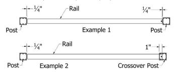
Crossover Railing: Cut bottom rail the same as (Example 1). For top rail, make end spacing exactly 1" longer on all ends connecting to line crossover post (Example 2). If connecting to a corner crossover cut top rail 1/4" short of post.
